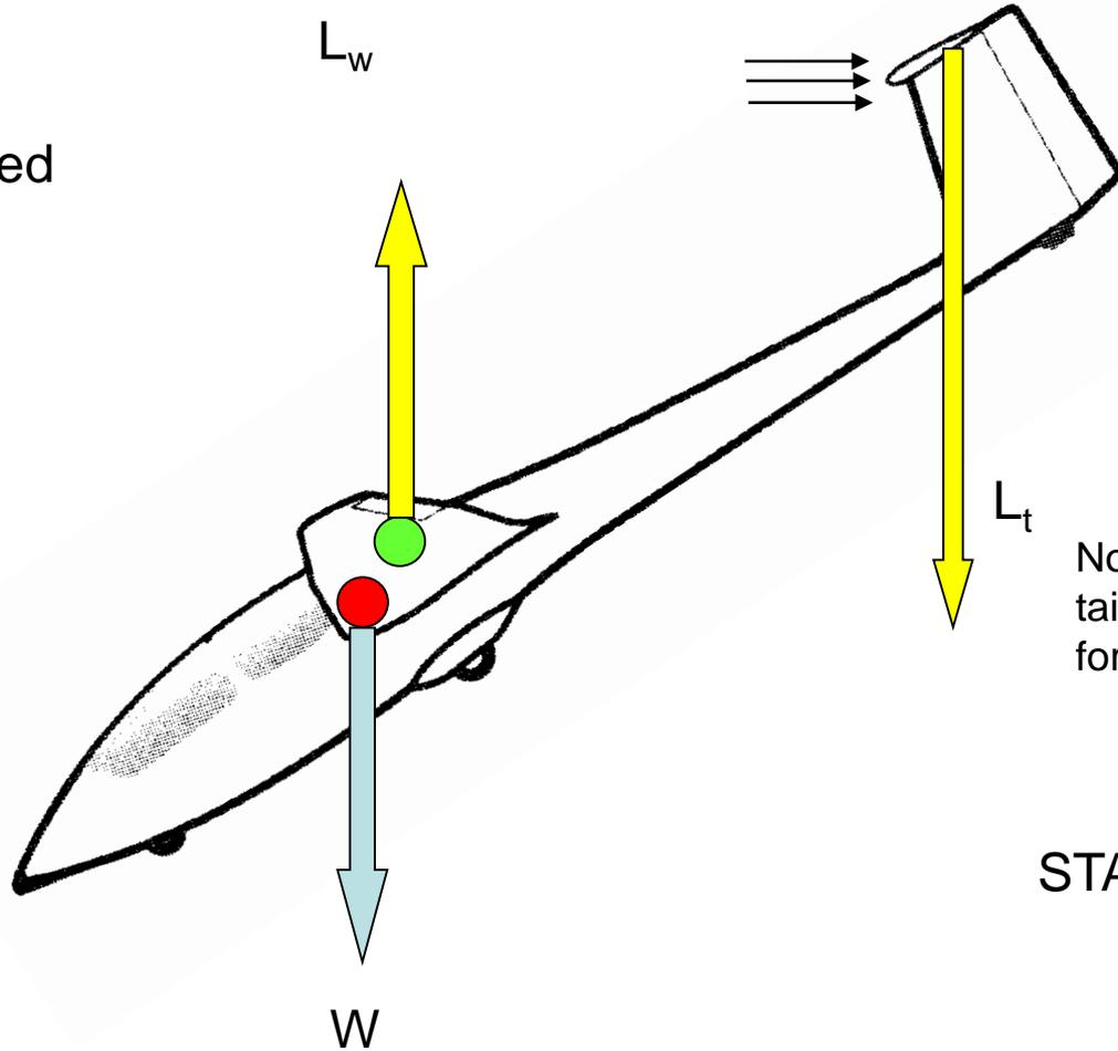
Note: The bigger the  $\alpha$  of the tail the bigger the restoring force
