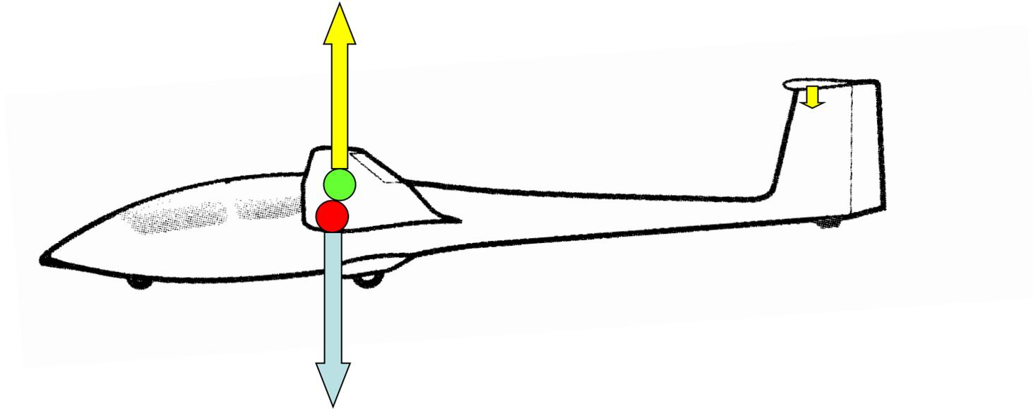
This is so that during a pitch-up the tailplane will continue to have a lower AoA than the main wing which will stall before the tail so still allowing use of the elevator to lower the nose for recovery.
