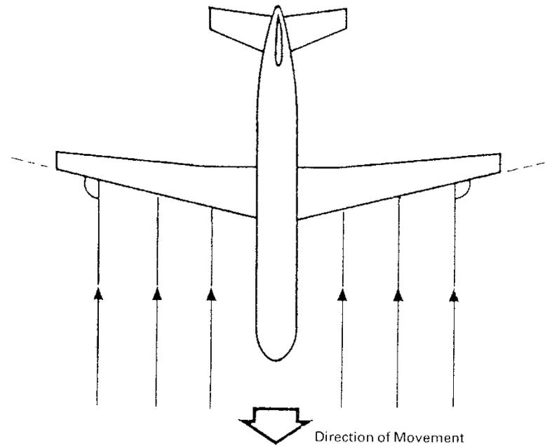
When airflow meets wings asymmetrically more lift is produced on one side tending to roll the aircraft level
