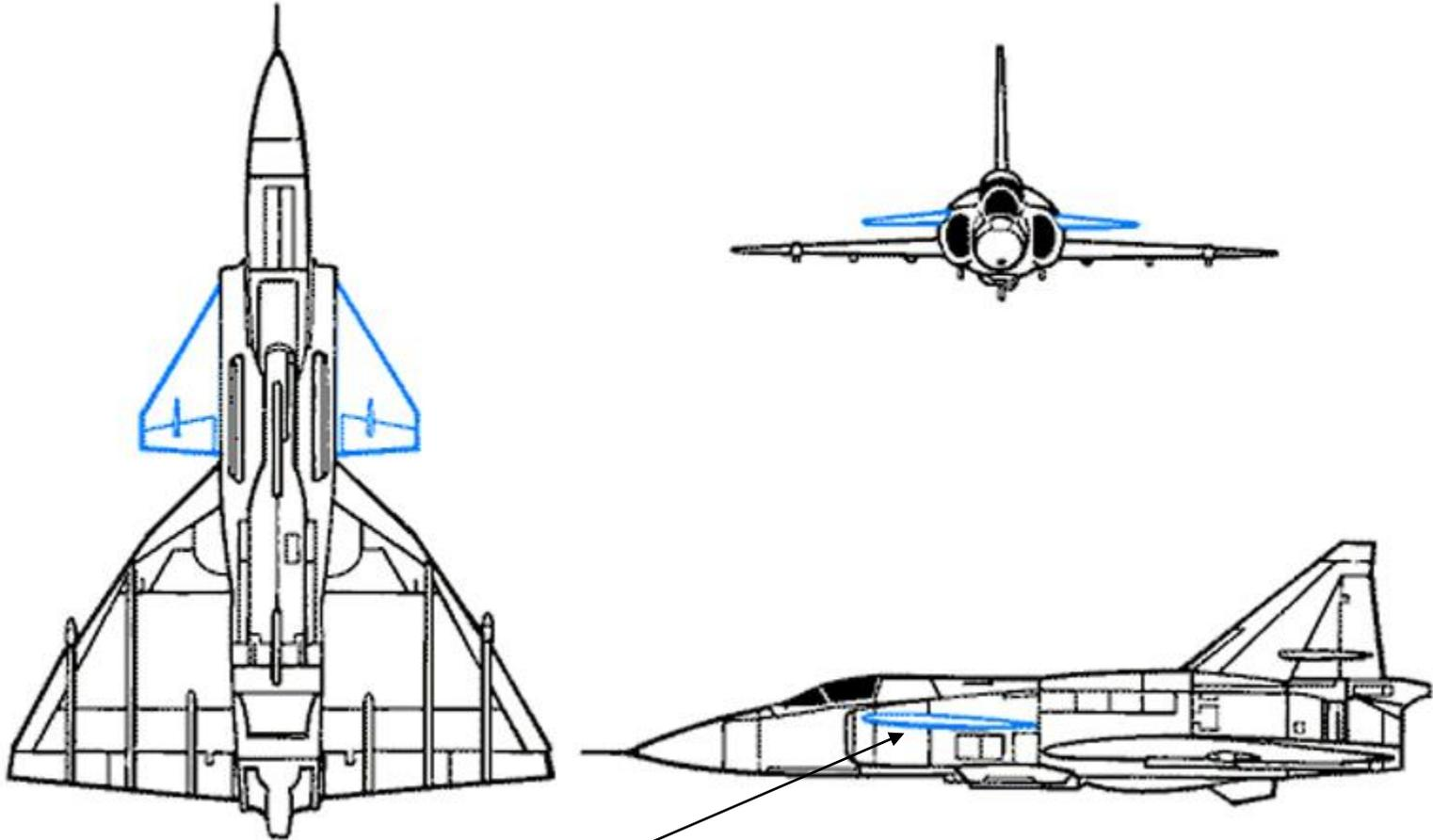
Canard reaches stall angle before main wing. Therefore stalls before main wing – nose goes down – stops main wing stalling.
